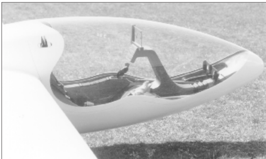
Glasflügel created this concept cockpit in 1981 which featured a heads-up liquid crystal display instrument panel. It looks good and the view is great, but there is not much pilot protection.
